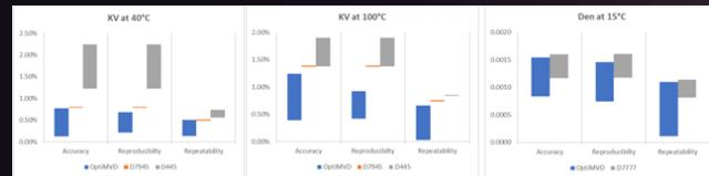
Figure 1: The accuracy, repeatability, and reproducibility of the OptiMVD as compared to ASTM D445 and ASTM D7945
